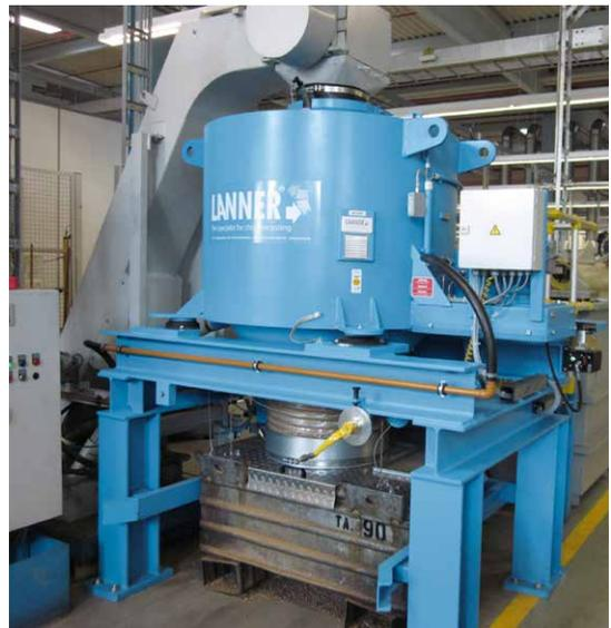
After 8 years of continuous work in 3-shift-operation the capacity of the perfectly working DS50 lifting bottom centrifuge was too small and therefore had to be replaced by the next bigger centrifuge of the same type.
