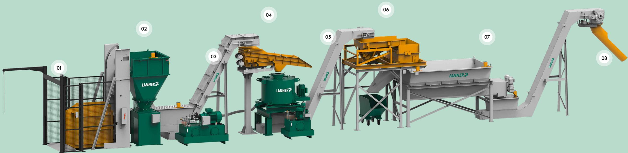
**01** Coolant containing chips are put through the chip cart into the hopper of the chip crusher by the chip cart dumper.
